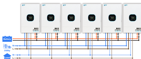
Parallel Operation in Single phase
